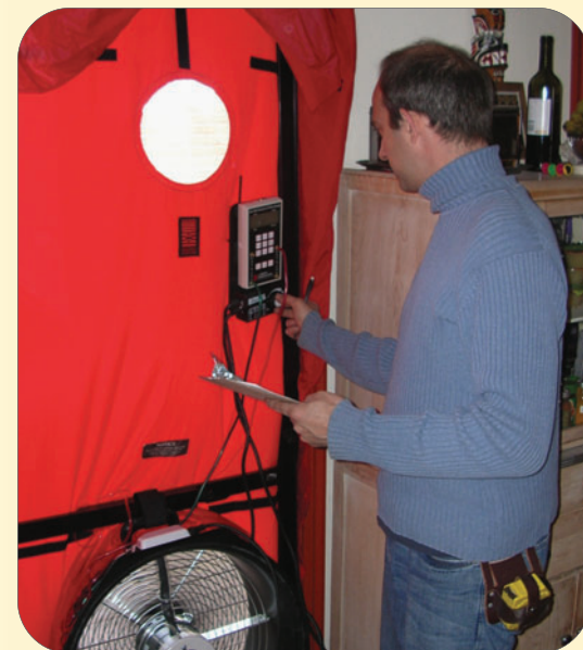
The EnerGuide service includes a blower door test, used to establish a house's energy efficiency rating.
