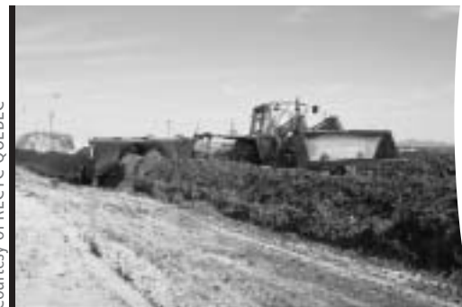
Returning of windrows on an outdoor composting platform
