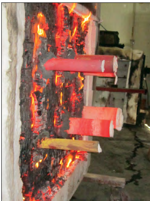
Figure 11 Fire stops penetrating cross-laminated timber and evaluated according to CAN/ULC S115 (Photo: Intertek)
