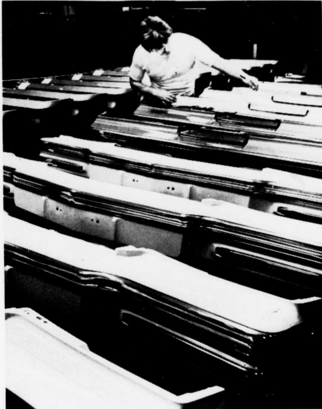
Taking weight out of passenger cars and trucks to improve fuel economy is an ongoing goal of General Motors. These new, lightweight polyurethane "soft face" front and rear bumpers together are 100 pounds lighter than the metal bumpers they replaced. They are noncorrosive and energy absorbing, compressing on low-speed impact and then returning to their original shapes. Painted to match car colors, they have bright metallic trim strips, also flexible to resist damage.
