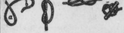
Fig. 1. (Fig. 1) is the simplest of all. It is made at the end of a rope, to prevent it passing through a hole, or to prevent the strands from separating too far.
