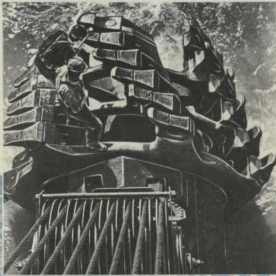
Mammoth 26-ton rotating cutter of the "HYDRO-QUEBEC," a dredge, equipped with renewable teeth.
