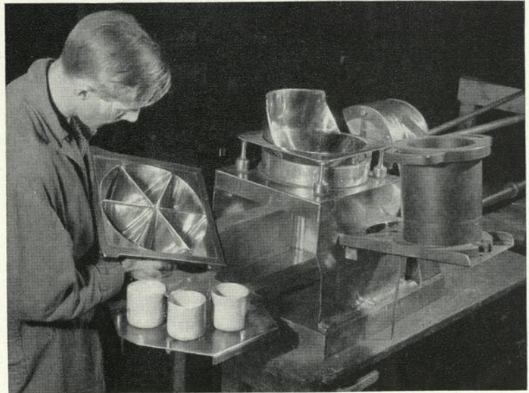
Above: Making apparatus for the manufacture of lead azide. Note the mirror finish essential on all appliances in contact with this super-sensitive detonating compound.
