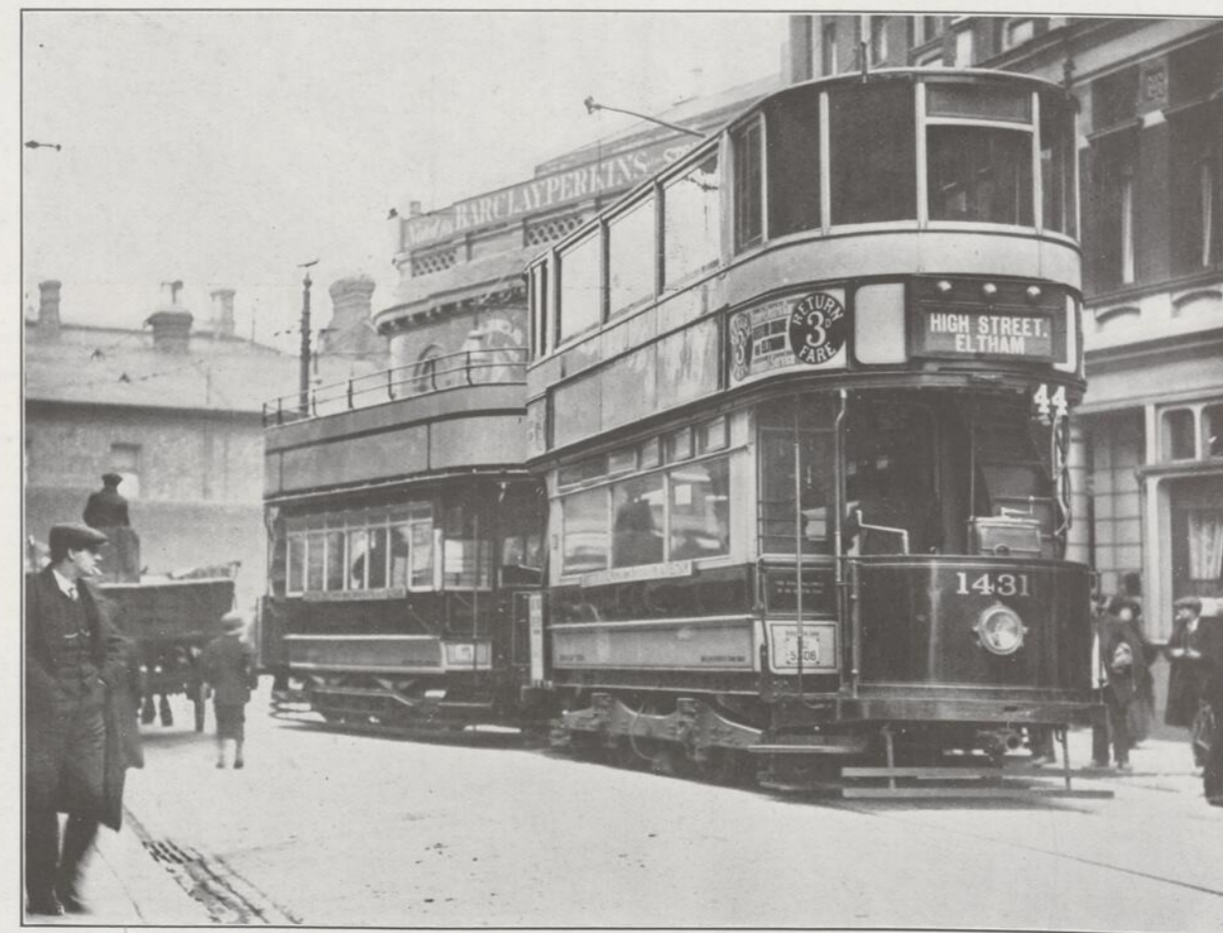
THE SOLUTION OF THE STREET-CAR PROBLEM IN MONTREAL—A double deck car such as that which was recently recommended to the Montreal Tramways Company for use on the streets of Montreal. In the above picture a trailer is attached to the car, both cars being used at the rush hours of the day to convey workmen to and from the Woolwich arsenal. It will be noted that the trailer is also double-decked. (Copyright Sports and General Press Agency)
