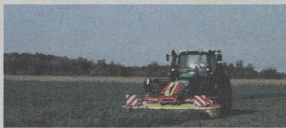
2014 Pottinger 351 ALPHA-MOTION Disc Mower "New" 3.46 M, excellent condition, 2014, FRONT DISC MOWER Behind the new "alpha-motion" front technology are the well-thought-out kinematics of the support frame. In contrast to "state-of-the-art" drawn rack systems, the support frame itself reacts to every unevenness of the terrain, as well as the connection rods. The mower unit is also raised when there is an incline and lowered for downhill slopes.
