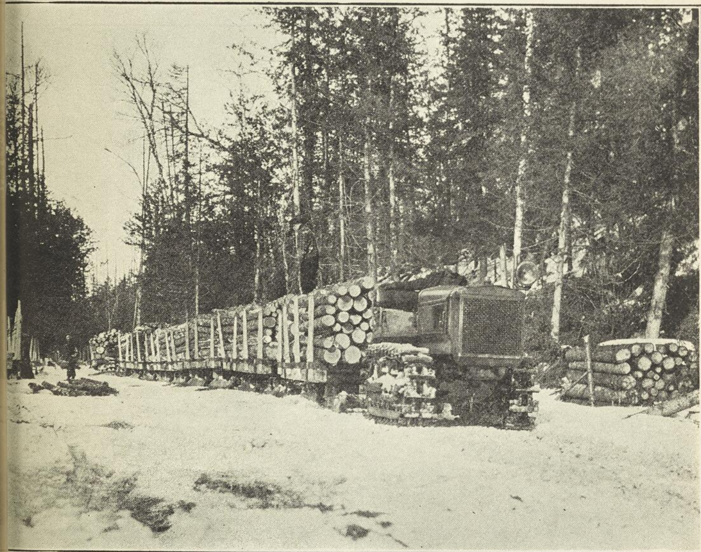
At the make up siding of the Provincial Pulp and Paper Co. They started their tractor work 4 years ago by buying 2 Fordsons. They junked these and now own 2-5 tons and 2 thirtys. This year with these machines they hauled 15,000 cords of pulp wood over a 4½ mile haul for $1.45 a cord. Picture shows Thirty starting for dump with 20 cords of wood.
