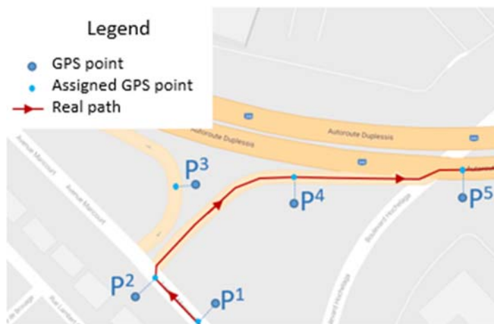
Figure 1. Incorrect assignment of point P 3 under the point-to-curve technique
