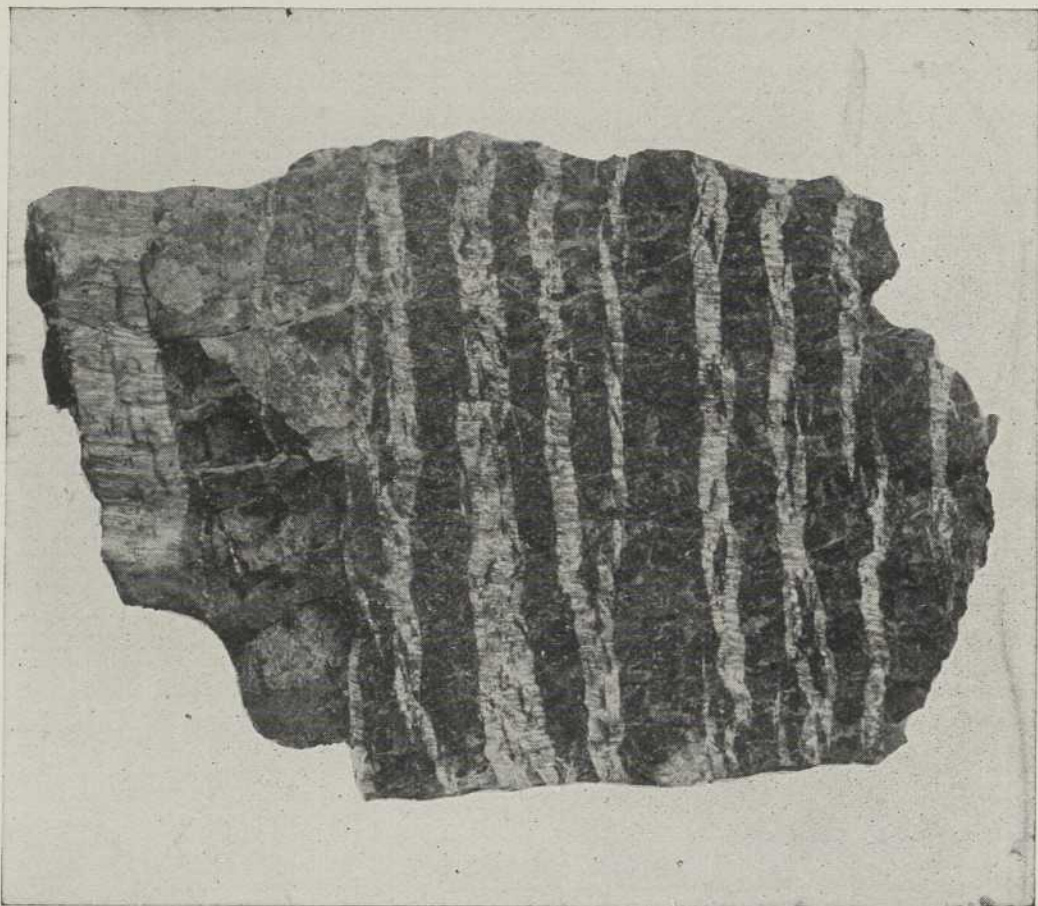
Asbestos rock, showing the banded or ribbon structure of the asbestos veins.
