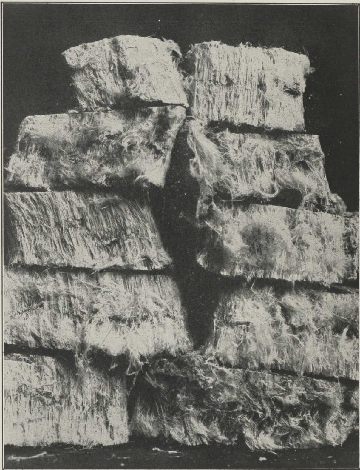
Chrysotile asbestos from Thetford Mines.—Quality “Crude No. 1”. Length of fibre 4\frac{1}{2} inches.
