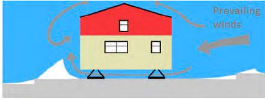
FIGURE 5.86: GENERAL RELATIONSHIP BETWEEN INFRASTRUCTURE AND SNOW COVER IN BUILT ENVIRONMENTS (FROM BOUCHARD, 2005).
