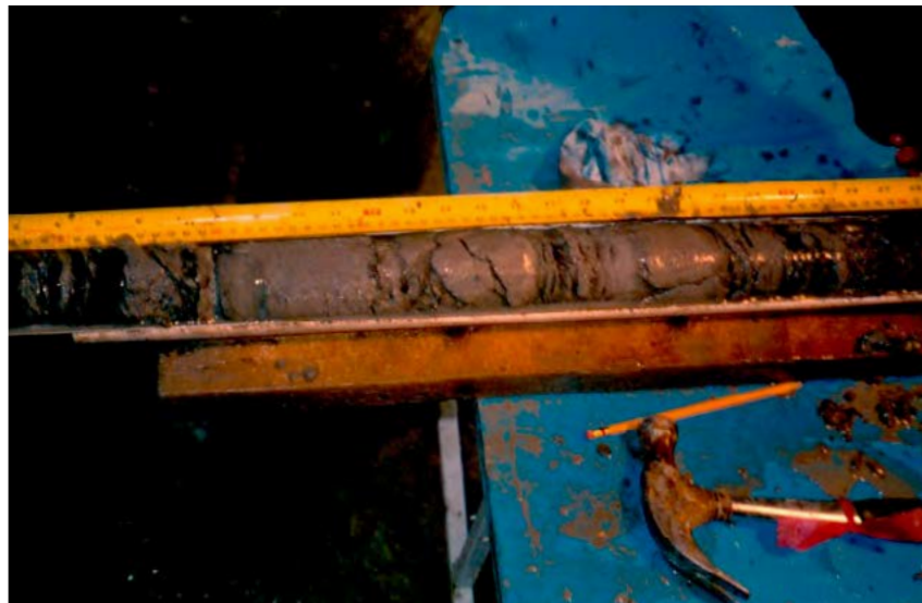
FIGURE 5.15: THICK ICE LENSES FORMED AT STRATIGRAPHIC CONTACTS BETWEEN LAYERS OF SAND AND LAYERS OF CLAY, AT UMIUJAQ.
