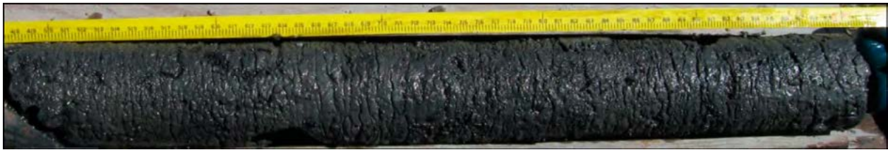
FIGURE 5.21: SEGREGATION ICE IN A HOLOCENE INTERTIDAL DIAMICT AT TASIUJAQ (UNDER THE AIRPORT RUNWAY).
