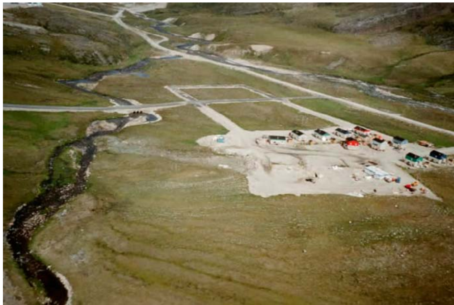
FIGURE 5.42: AN ACTIVE LAYER STRIKE-SLIP SLIDE AT SALLUIT IN 1998 RESULTED IN ABANDONMENT OF DEVELOPMENT OF THE NEW RESIDENTIAL NEIGHBOURHOOD AND THE MOVING OF SOME TWENTY RECENTLY INSTALLED HOMES.
