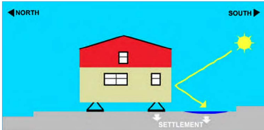
FIGURE 3.14: EFFECT OF PALE-COLOURED REFLECTIVE SIDING ON PERMAFROST. SOURCE: TOPOCLIMAT ET MICROCLIMATS DE LA VALLÉE DE SALLUIT (NUNAVIK), THESIS SUBMITTED TO THE FACULTY OF GRADUATE STUDIES, UNIVERSITÉ LAVAL
