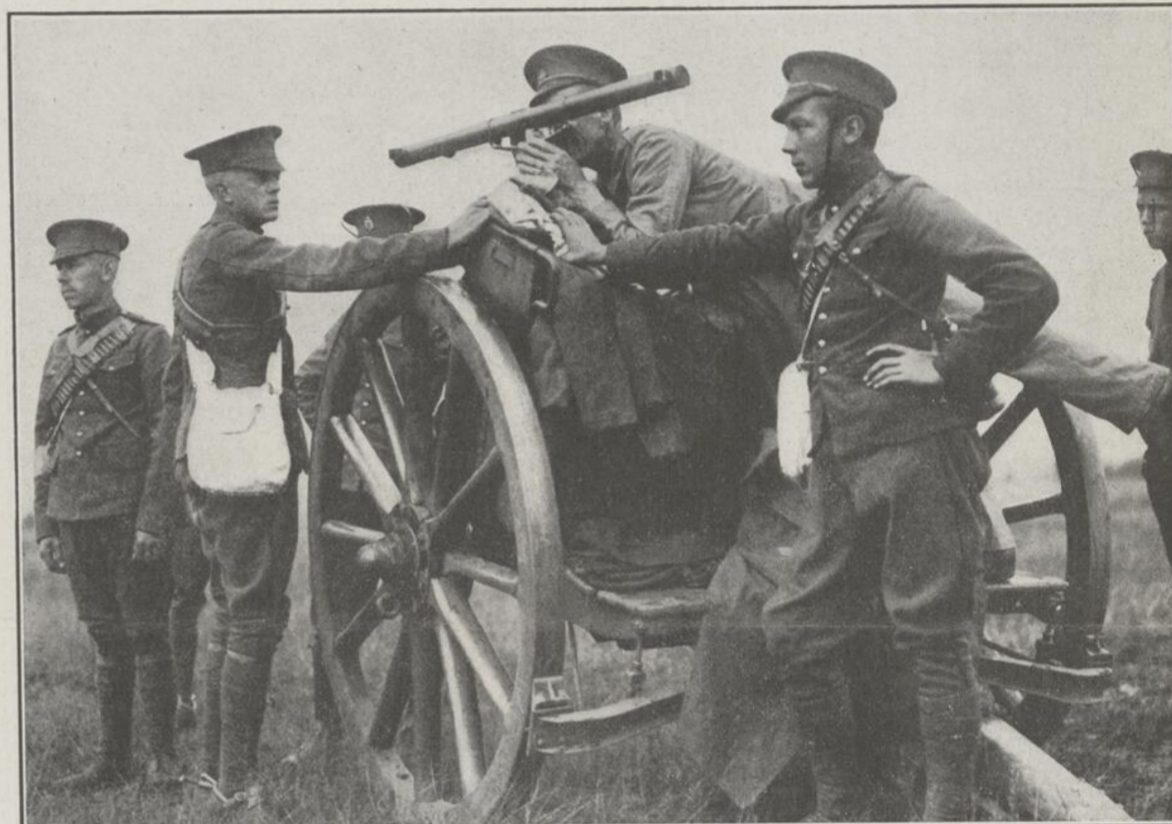
FINDING THE RANGE BEFORE LOOSENING THE DEADLY SHRAPNEL —With instruments such as that shown in the above illustration the Canadian artillery lads will be able to find the range of the enemy on their arrival at the front.
