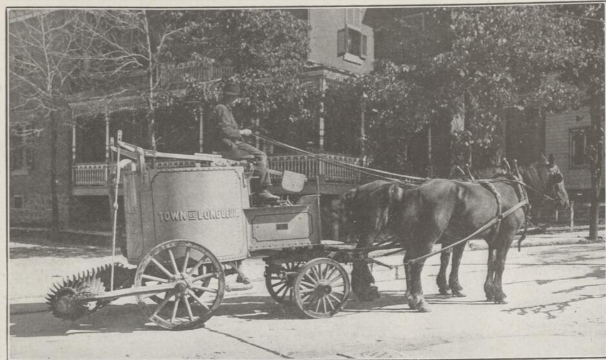
UP-TO-DATE LONGUEUIL—A combined watering cart and sprinkler, one of the new additions to the municipal cleaning plant of this historic old town. Longueuil has taken the lead in introducing this machine into the East. Several, however, are in use in the United States and Western Canada.
