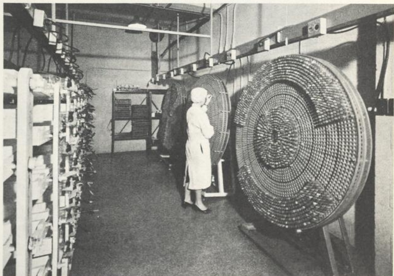
Tubes of tissue cultures and virus cultures are agitated by rotation.
