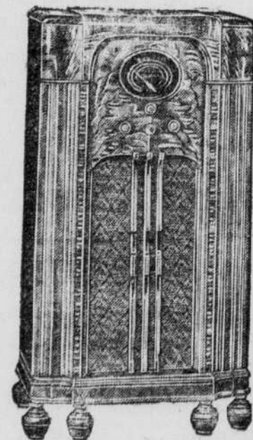
MARCONI MODEL 82 A.C.—8 Marconi RVC Radiotrons (1 metal, 4 glass) give continuous all-wave reception from 18.5M to 568M. Cathode ray tuning indicator. Glass dial with selective band illumination. Low tone booster. 12" dynamic speaker. AVC. Walnut sides flow outward to give beauty to recessed grille. Gorgeous front panel and raised top have moderne effect. Cabinet dimensions: Height 39 1/2", width 23 1/2", depth 13 1/2". Price $127.00
