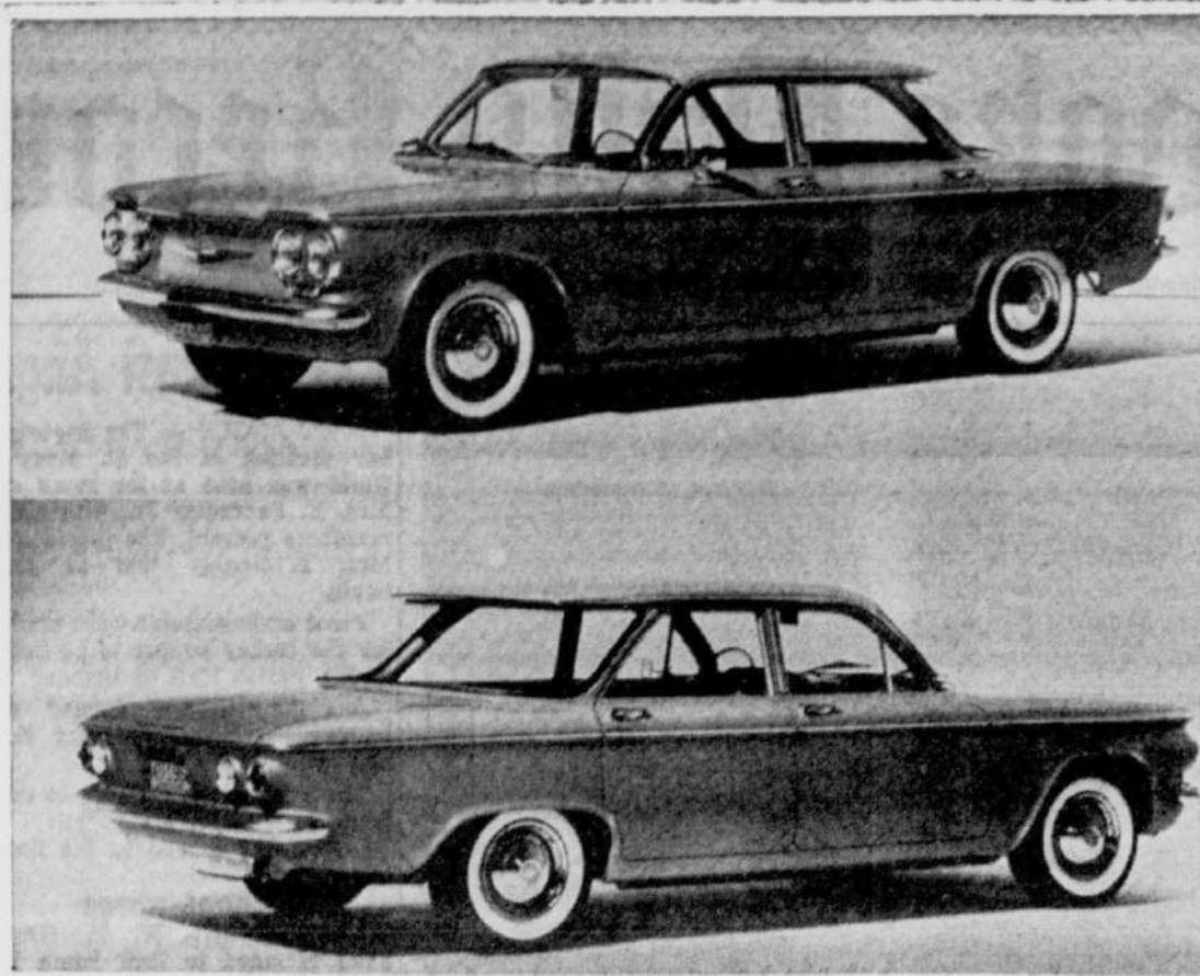
CHEVROLET CORVAIR — These two views of the new compact Chevrolet Corvair show its excellent all-around visibility, smooth styling and sleek appearance. The Corvair is only four feet three inches high and 15 feet long, yet it accommodates six people with ease. A light-weight air-cooled engine in the rear, independent four-wheel suspension system and unitized construction of frame and body are innovations.
