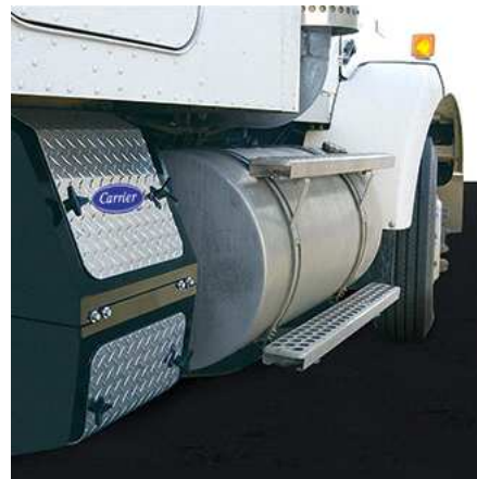
(b) Auxiliary Power Unit
