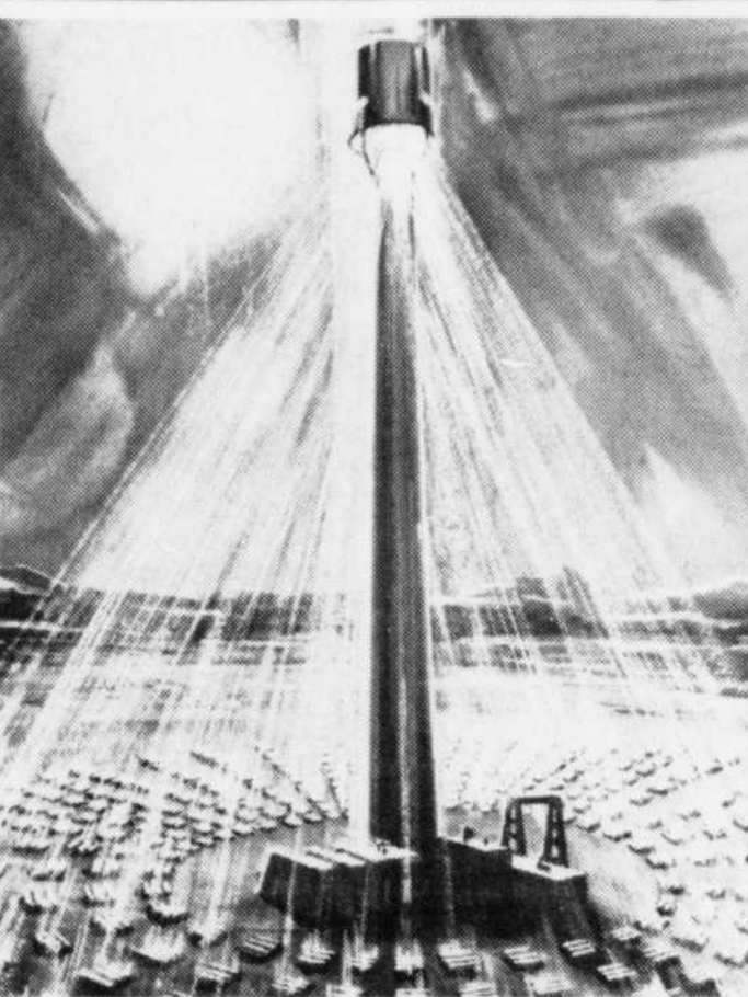
TOWER OF POWER under study as a possible new source of electricity would utilize computer-aimed mirrors to focus the sun's rays on a boiler atop the tower. Water converted to high-pressure steam would be pumped to a conventional steam-turbine generator at the tower's base. Research on the tower authorized by the Energy Research and Development Administration is being done by Honeywell solar energy scientists in Minneapolis.
