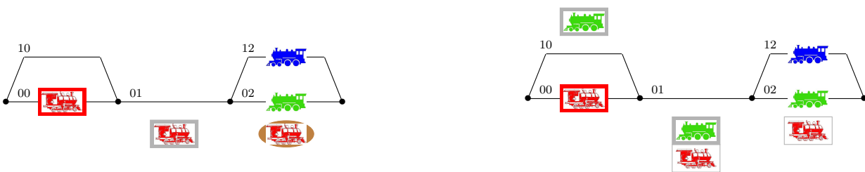
Figure 8: The red train requests to move. At the stage of the reservation process represented on the left diagram, the green train has to trigger a process (the red train is circled with brown because its reservation is not yet completed). So the reservation of the green train is placed in the first position of Section 01, by Rule 3 and leads to the right diagram.
