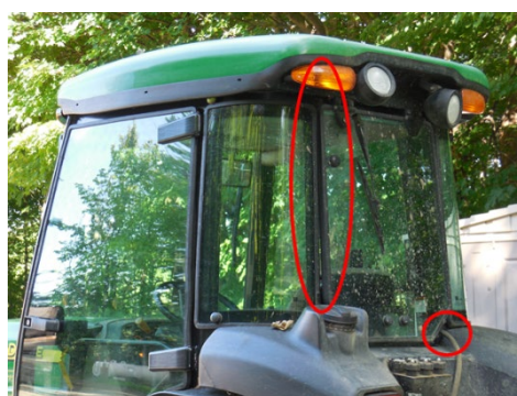
Figure 5. Tractor cab with openings
