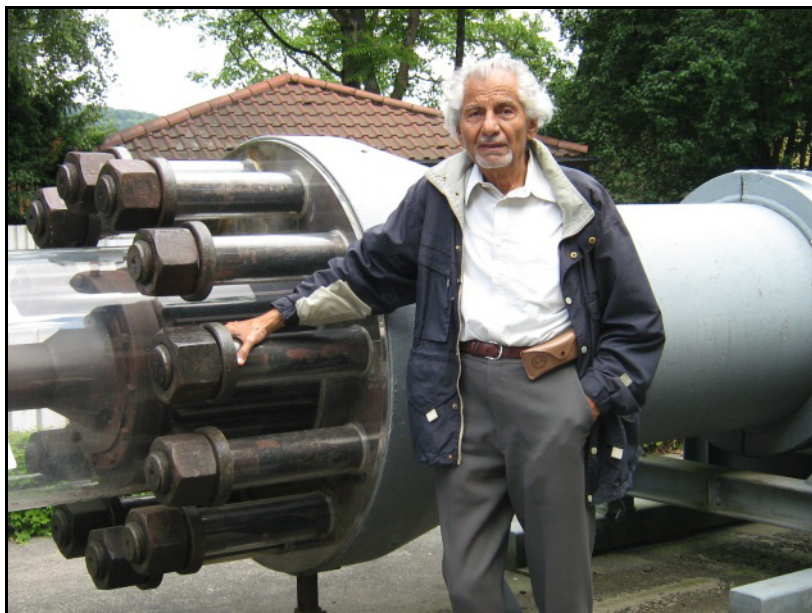
Figure 6.36: Example of high pressure reactors [photo by Nadia Habashi, 2009].
