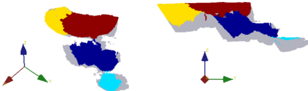
Figure 8: Phase seeds with non-mineable shapes (grey) that are to be added
