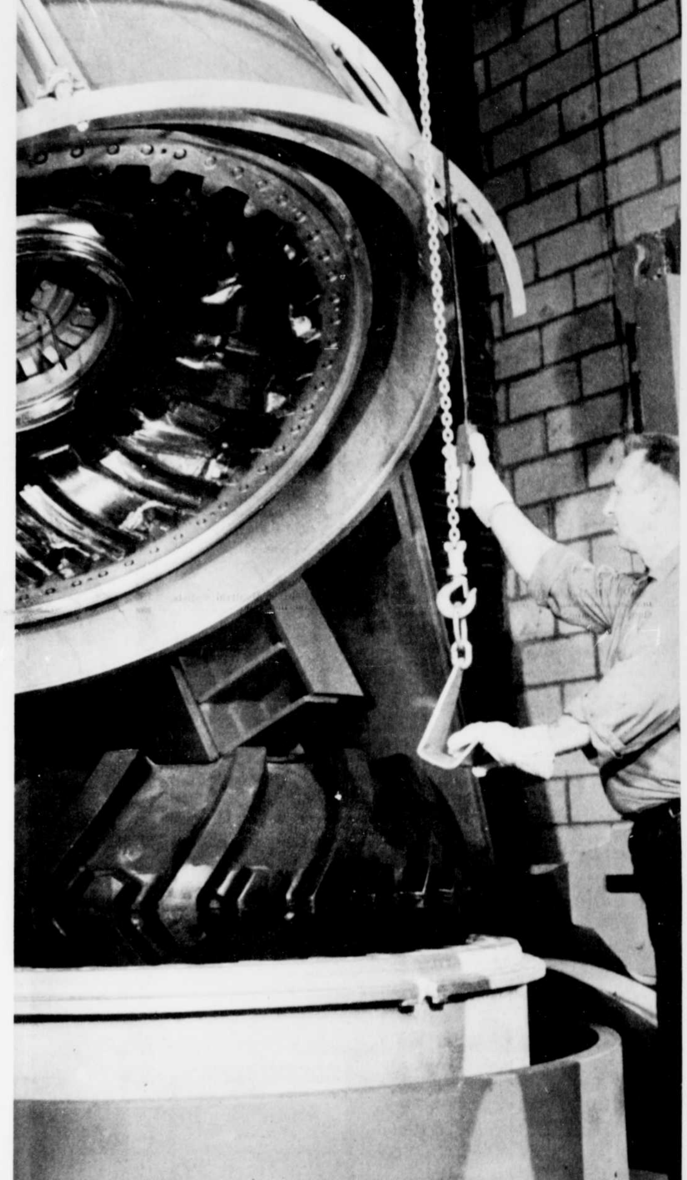
WITH A SNOWTIRE LIKE THIS... — About to be taken from mold at Toronto plant is Goodyear's newest tire for the logging industry: Called the Timber Torque Steelguard tire, it is reinforced with two layers of steel wire under the tread, which virtually eliminates punctures. This tire is more than six feet in diameter and weighs about half a ton.
