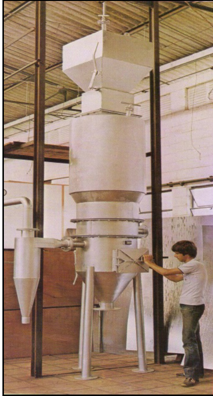
Figure 6.7: Wood gasification unit.
