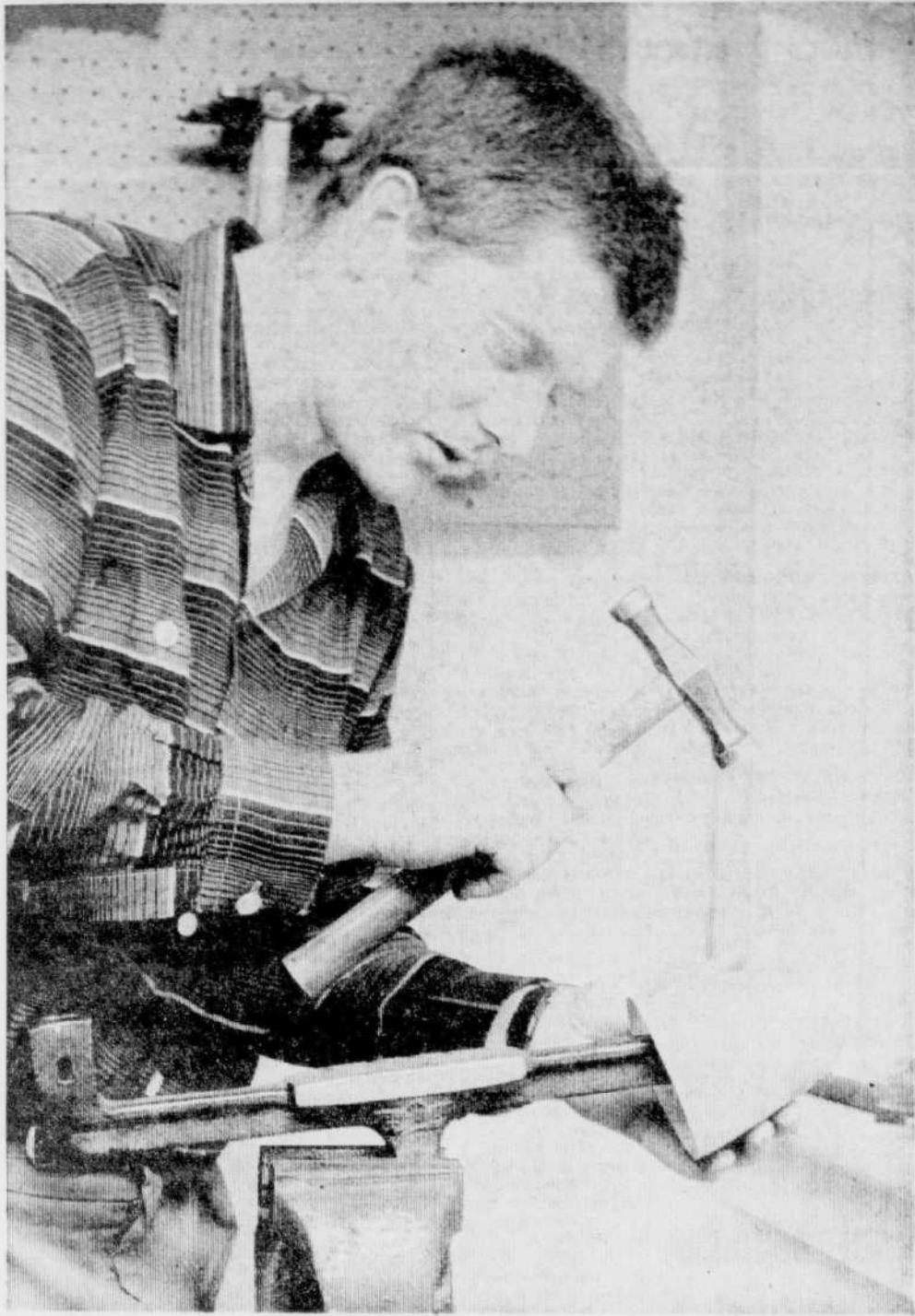
FORMING THE CUP — Marc Beaudoin, North Hatley silversmith, fashions a chalice using an anvil and a raising hammer. Mr. Beaudoin never uses machinery in his work and as result each chalice takes at least 10 days to complete. (Record Photo by Doug Gerrish)
