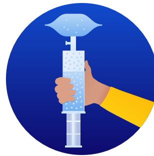
Indirect measurement by extracting dissolved gases using the headspace technique or an automated system
