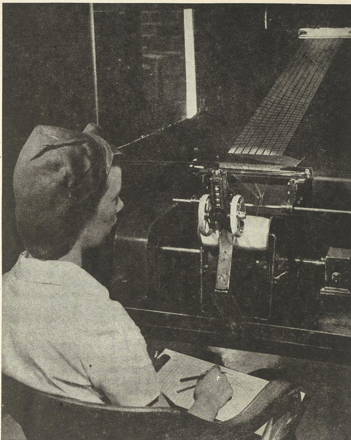
FIG. 1. The operation on which this girl is working is called the creel mirror test. Most nylon yarn is composed of a group of filaments and when one or more is broken it can be seen easily in this machine. Yarn from 40 separate packages is being drawn at the rate of 25 yards per minute through a cabinet where the yarn only is brightly illuminated. The operator keeps a record of the number of defects while winding off 1,000 yards. It is not unusual to find no defects whatever, and seldom does the level exceed 0.5 defects per thousand yards, that is, 20 in the 1,000 yards from each 40 packages.
