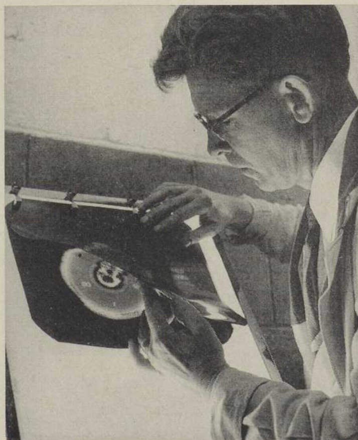
X-RAY INSPECTION OF WELDS TURNS UP INTERNAL FLAWS.
