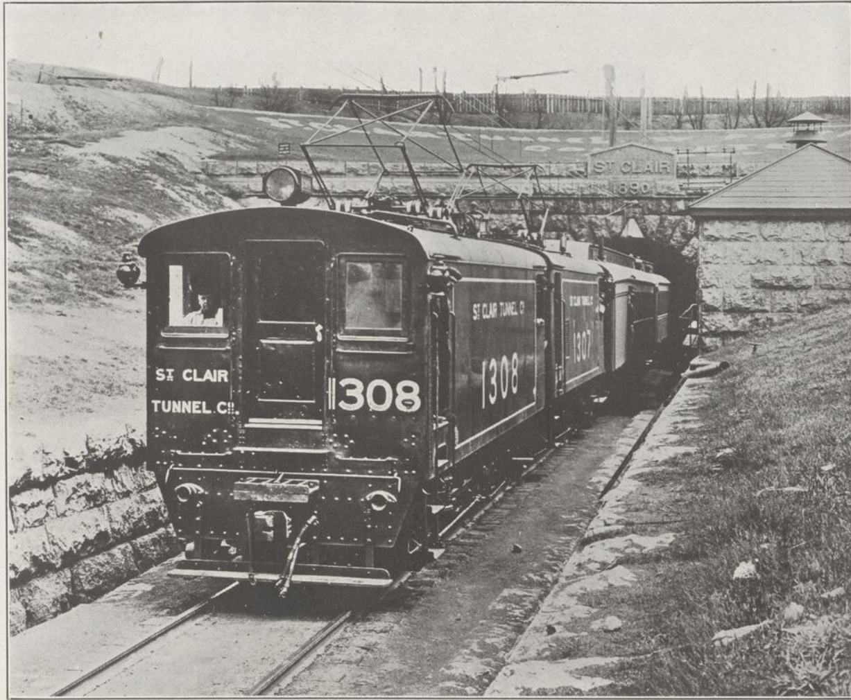
THE ELECTRIFICATION OF THE ST. CLAIR TUNNEL—An electric locomotive hauling a Grand Trunk passenger train out of the tunnel, which extends under the River St. Clair from Sarnia, on the Canadian side, to Port Huron on the United States side. Until a couple of weeks ago trains were hauled through the tunnel by powerful steam locomotives, but the deadly fumes and gases generated by these made it necessary to install electric locomotives. (Photo by courtesy of the G.T.R.)
