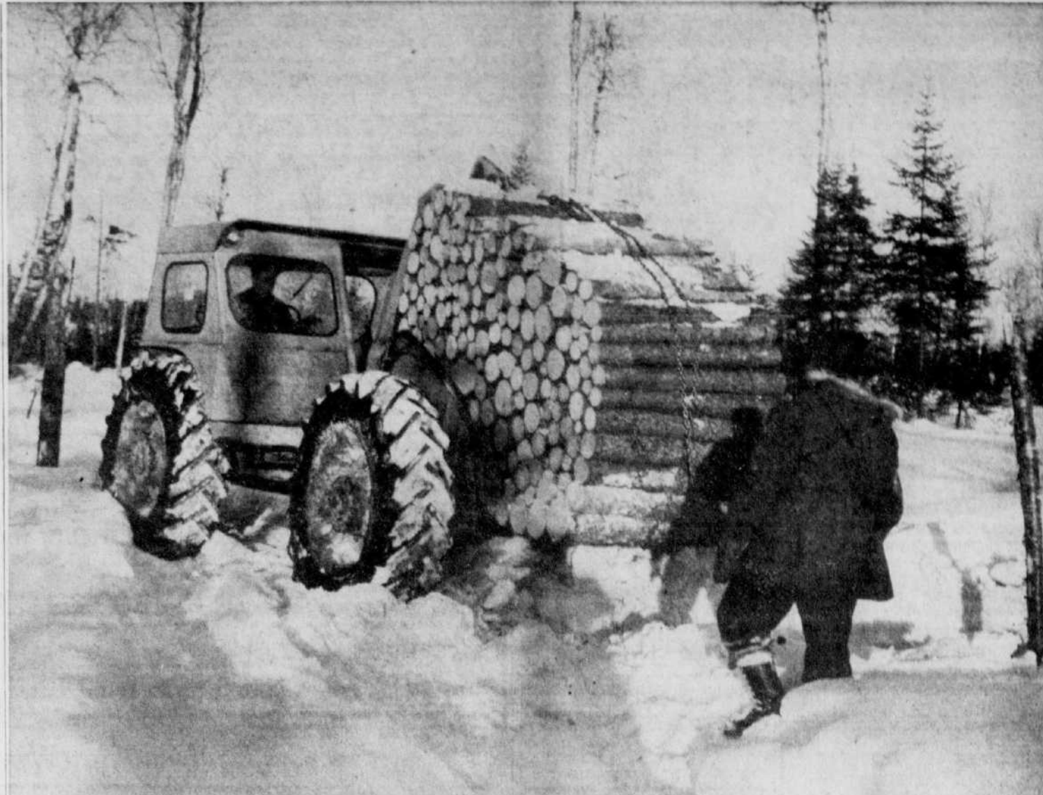
Mechanical Logger — A new mechanical logger is at work in the woods of Ontario and Quebec. The machine shown here was built by the woodlands section of the Canadian Pulp and Paper Association and five of them are in experimental use. The machine, which has four-wheel drive, can pick up 3½ tons of pulp-wood logs, transport them across the roughest woodland terrain and dump them wherever they are needed. (CP)
