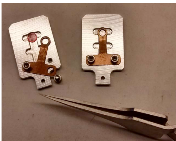
Figure 8 – Aluminum microscopy grid holder
