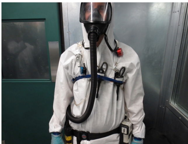
Figure 6 – Arrangement of personal sampling devices on a worker.
