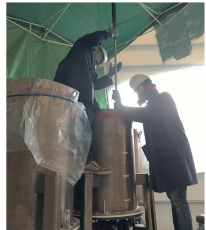
Soil core sampling during a controlled dilbit spill
