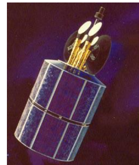
Satellite de communication Intelsat IV.
