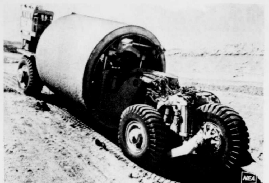
MOVING BETTER, ELECTRICALLY. Carrying and accurately positioning 150-ton, 20-foot-diameter sections of concrete pipe is an easy task for this electrically driven "Pipemobile." Equipped with a GE transmission with a 1,500-horsepower four-wheel drive, the machine is placing pipe for a water line in southern California. A unique feature of the 21-foot-high, 64-foot-long pipe transporter is its modular design. When the six-mile-long pipeline is completed late in 1970, the machine can be quickly disassembled for transport to another site and easily reassembled there.
