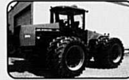
Case IH 9250, 4RM, cab., 1993, 5911 h, 6 cyl. trans. 12 vit. power shift, 4 valves hyd., force 300 PTO, pneus arrières : 20.8 x 42 dual Firestone, roues dbles, barrage diff., attelage 3 pts.
