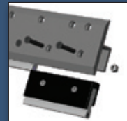
Front view of one wearing edge removed
