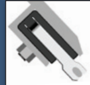
Side view of wearing edge and rubber housing
