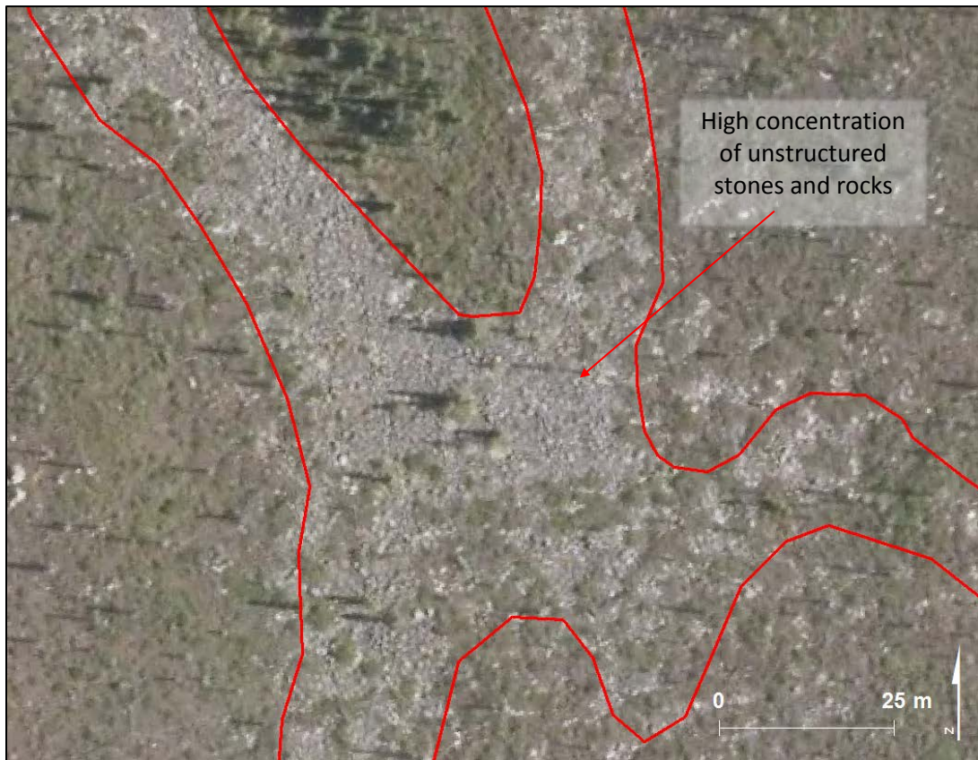
Figure 9. Example of a glacial block field (1ab), on an aerial photograph, in the Western Spruce-Moss ecozone
