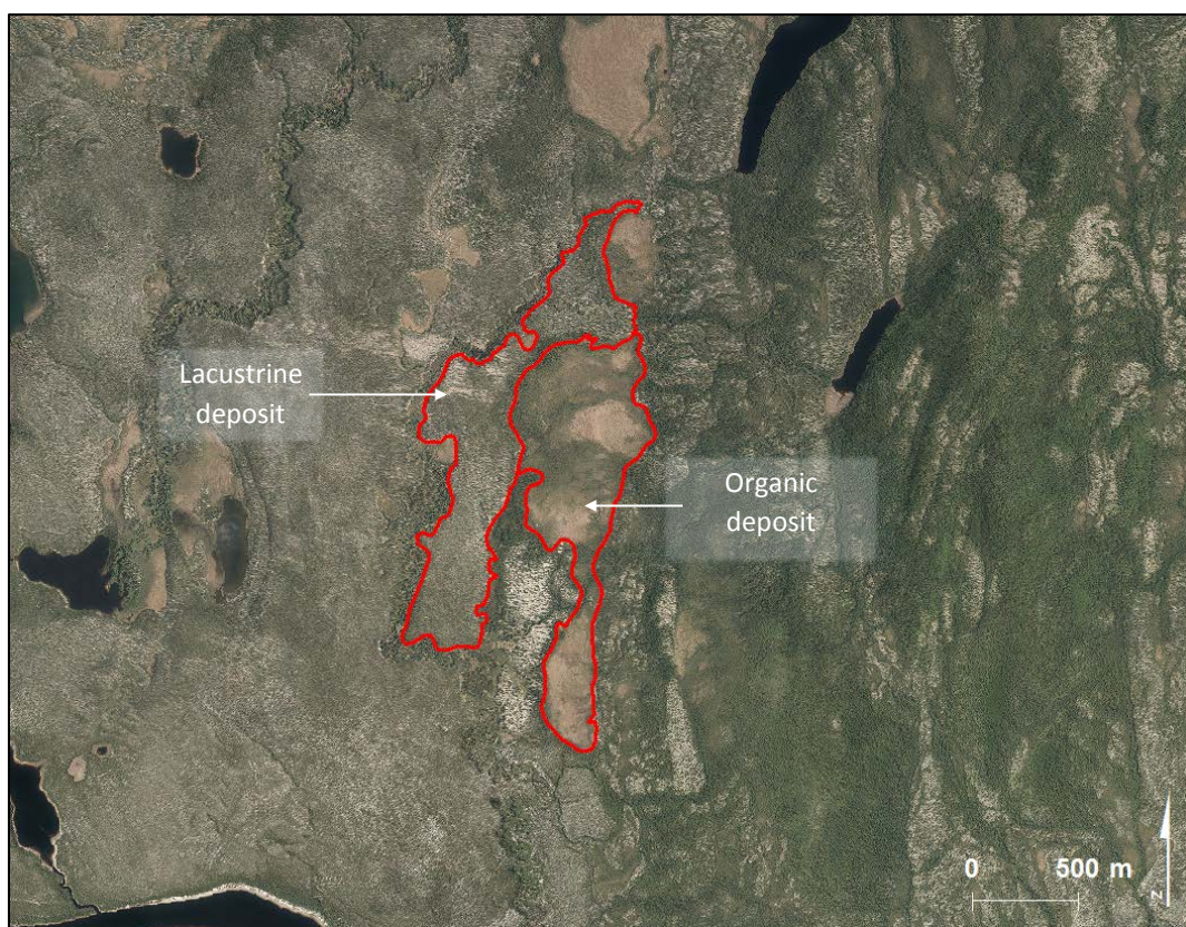
Figure 68. Example of an organic deposit adjacent to a lacustrine deposit, on an aerial photograph, in the Western Spruce-Moss ecozone
