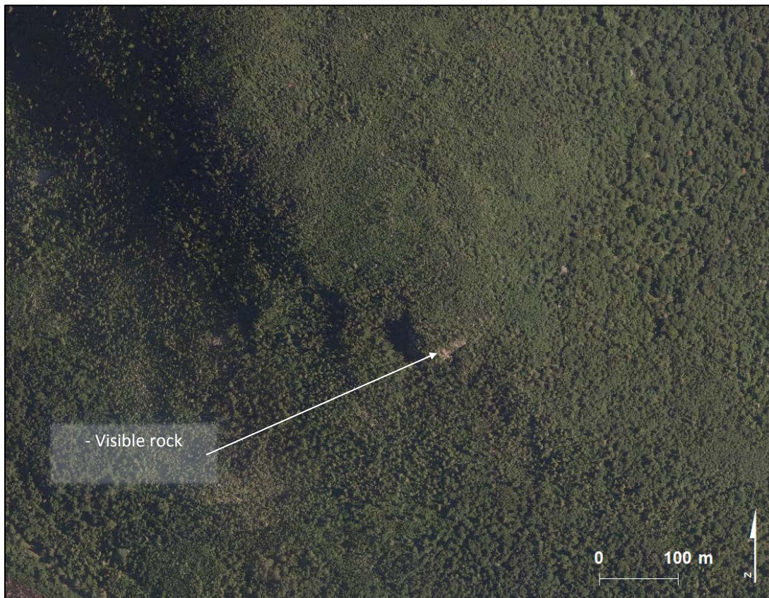
Figure 6. Example of very thin till (R1a), on an aerial photograph, in the Eastern Balsam Fir- White Birch ecozone
