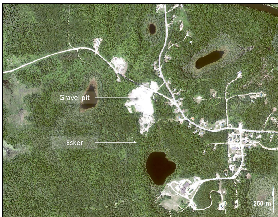
Figure 51. Example of an esker under a lacustrine deposit, on an aerial photograph, in the Western Sugar Maple-Linden ecozone
