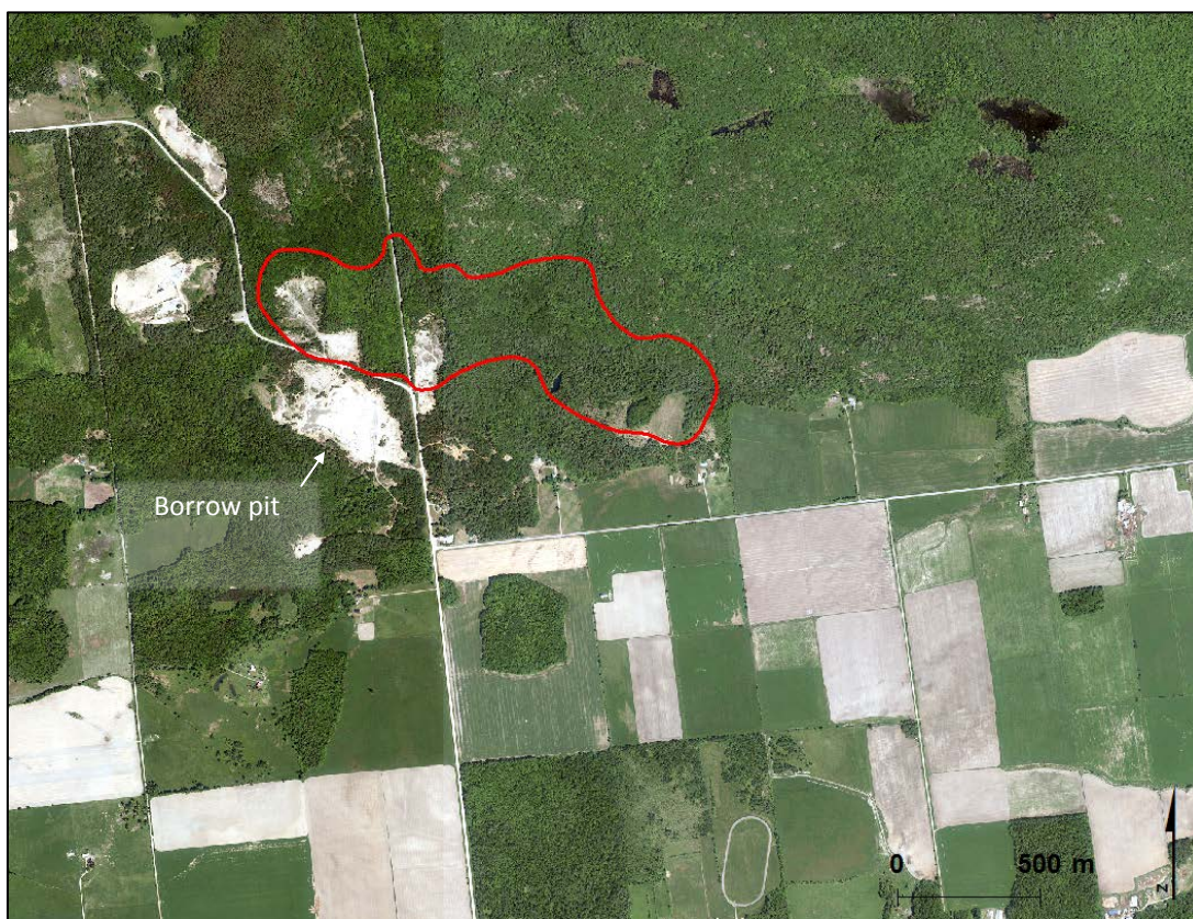
Figure 63. Example of a raised beach (6s), on an aerial photograph, in the Sugar Maple-Butternut Hickory ecozone
