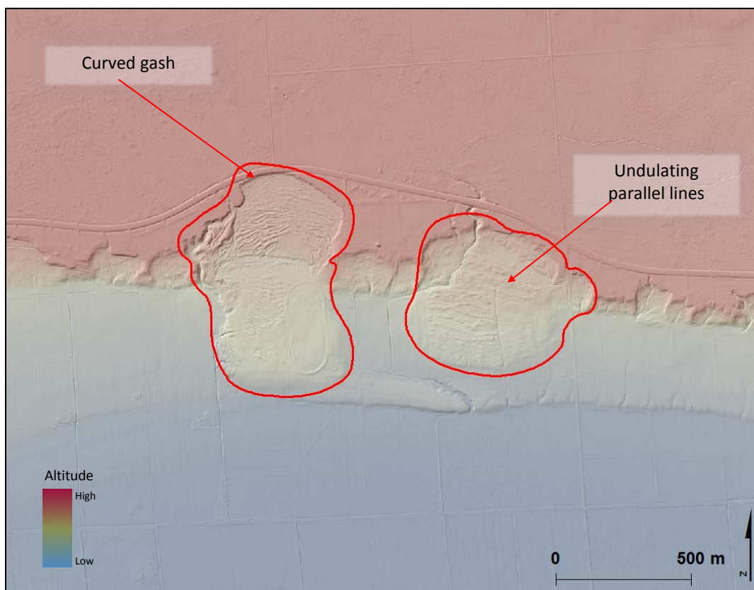
Figure 75. Example of a landslide (8g), on LiDAR, in the Sugar Maple-Butternut Hickory ecozone
