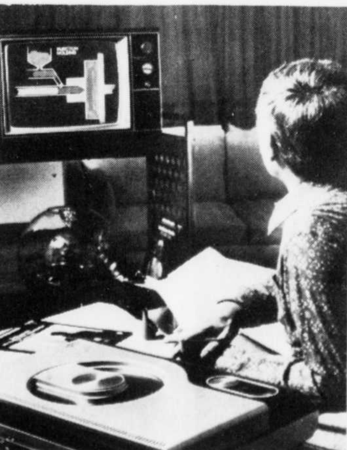
SPACE AGE GIZMO on table beside TV viewer is called a videodisc system which "plays" a grooveless record by laser beam and projects a video image, accompanied by a soundtrack, on any modified TV set. This revolutionary entertainment device will be available to the public next year. Also available will be over 200 discs offering movies and musicals.
