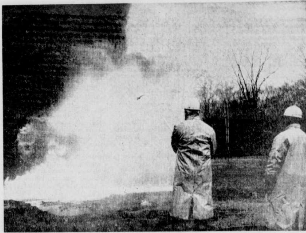
FOG PUTS IT OUT — Spray from a fog nozzle fire hose turns into vapor and smothers a demonstration fire yesterday at Victoria Park. Manning the hose is Andre
