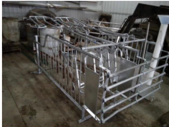
Figure 6 First prototype assembled in a factory (antenna and feeding system not assembled on this picture)
