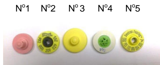
Figure 10 Tags tested with the Gestal RFID
