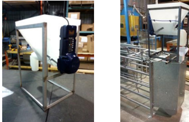
Figure 47 Feed reserve and Gestal system that can easily be removed from the base of the feeding station
