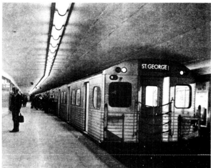
Train of aluminum subway cars similar in design to 164 now under construction for Toronto Transit Commission by Hawker Siddeley Canada Ltd. Lighter and larger than TTC's steel cars, they provide savings around 20% in power and maintenance costs.
