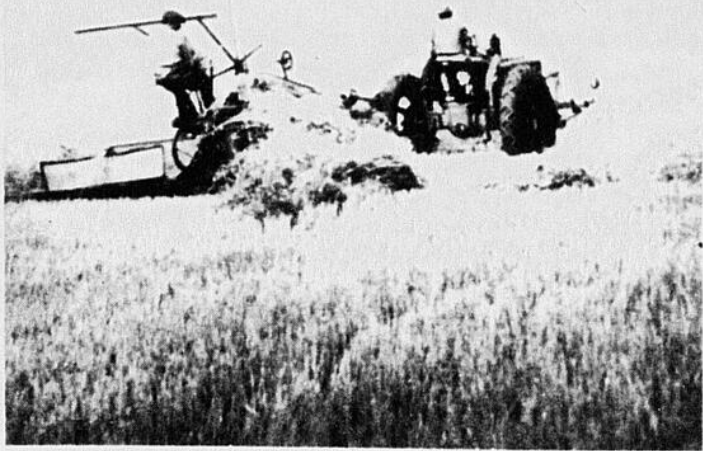
Remember when the binder attachment to the reaper first came into use? It saved many man hours previously required to bind the cut grain in preparation for threshing.
