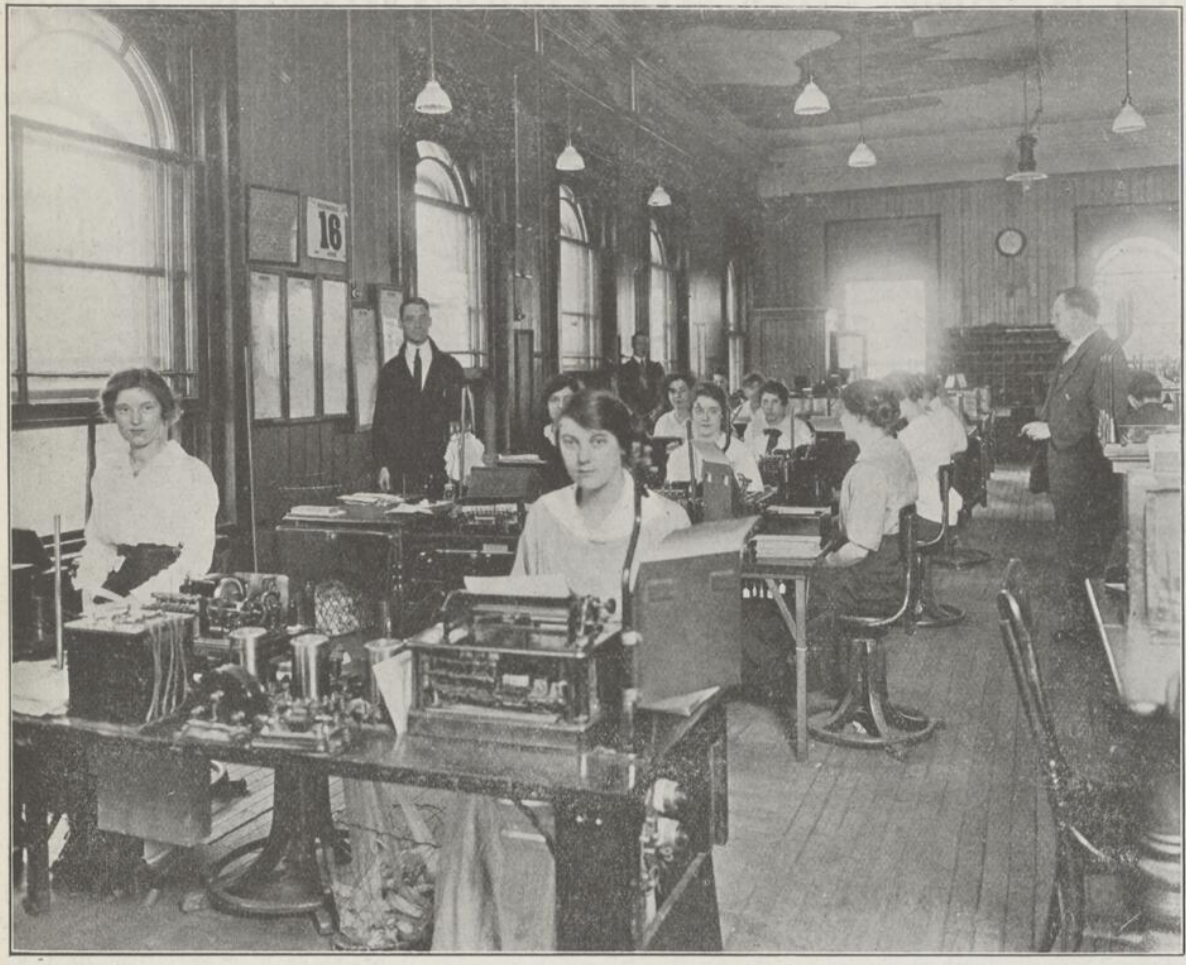
MODERN TELEGRAPH EQUIPMENT. THE INTERIOR OF THE PRINTER DEPARTMENT OF THE G.N.W. TELEGRAPH COMPANY, MONTREAL.—The machine shown in the above picture transmits telegrams at a very high speed between Montreal and principal Canadian and United States points. The messages come out on the distant end automatically typed on a telegraph blank ready for delivery.
