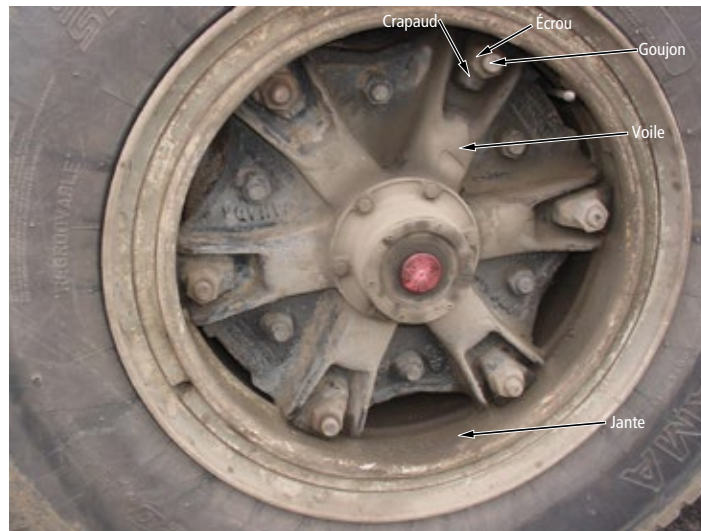
FIGURE 45 | Roue moulée ( spoke wheel )
