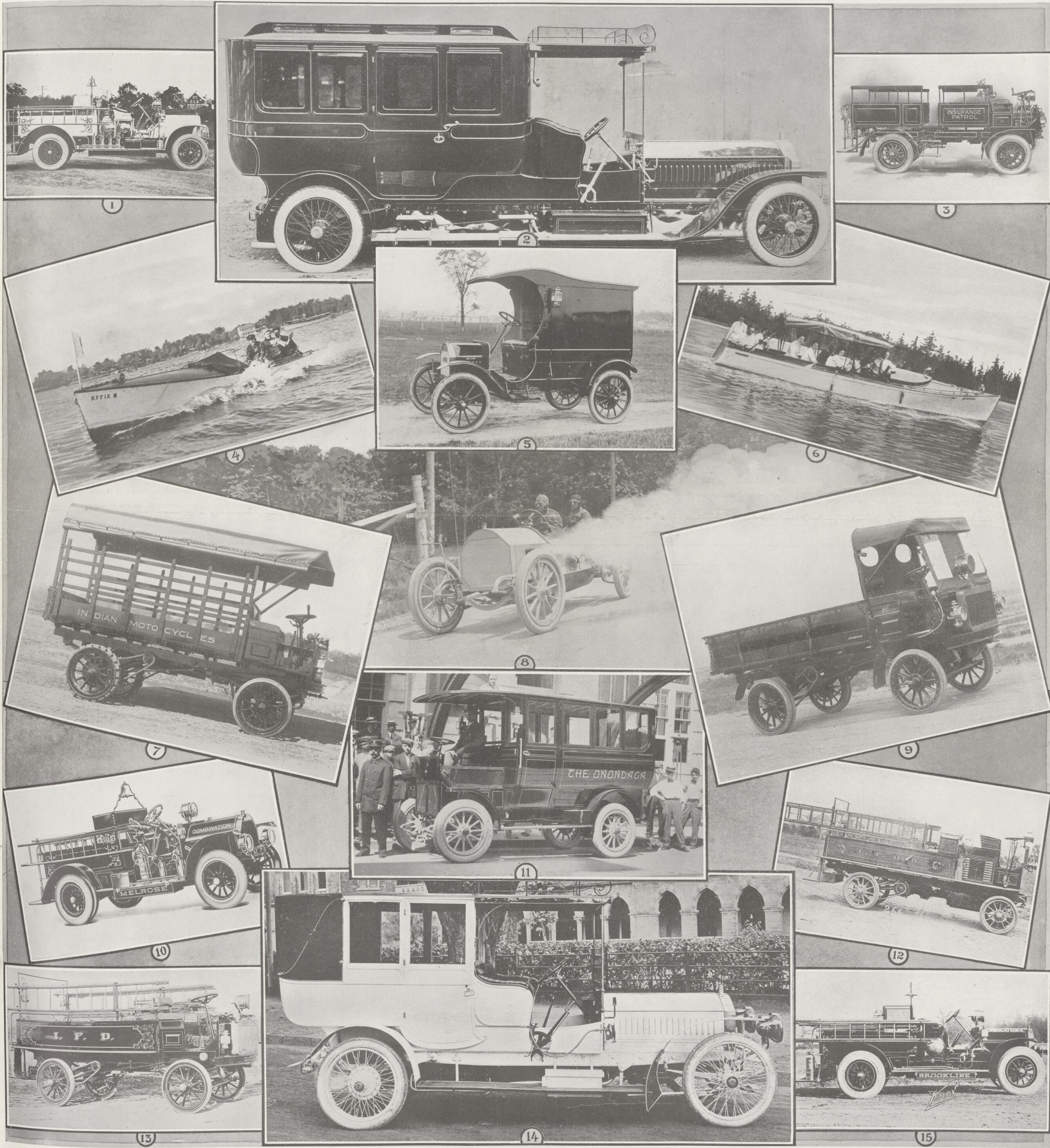
UNIQUE SERIES OF PICTURES ILLUSTRATIVE OF THE DEVELOPMENT OF MOTOR TRANSPORTATION—(1) Combination chemical engine and hose wagon. (2) The largest and most powerful private motor carriage in the world (a 90 h.p. 6-cylinder Napier, 120 brake horse-power, capable of carrying 12 persons); it was made in India for the Nizam of Hyderabad. (3) An insurance patrol. (4 and 6) Motor boats fitted with up-to-date marine engines. (5) A delivery wagon. (7) A motor truck. (8) A racing car going at full speed. (9) Another type of motor truck. (10, 12, 13 and 15) Different types of combination chemical engines and hose wagons. (11) A motor bus. (14) Another six-cylinder noiseless Napier car, built in India for one of the Indian potentates. The bodies of the Indian cars were made in India by local coach-builders. Both cars are luxuriously fitted up.
