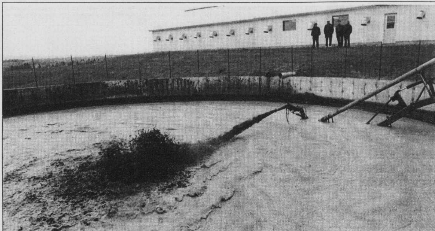
A powerful pump stirred a sloppy slurry of prime pig poop into the texture of heavy cream,
