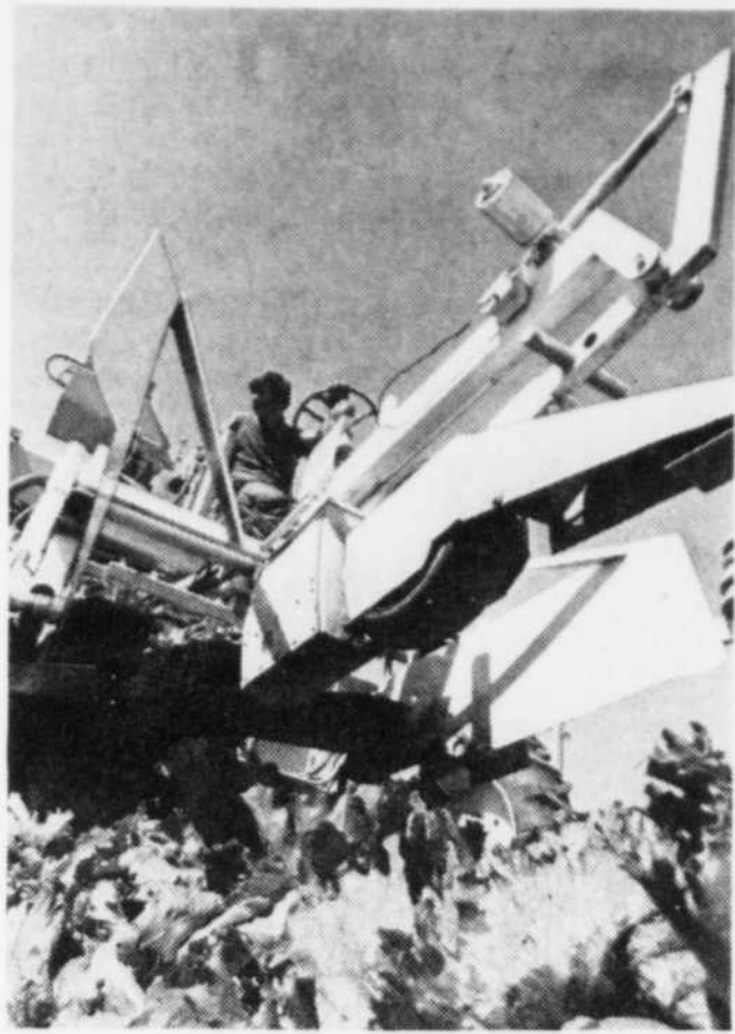
BETTER LETTUCE through X-rays is the idea of an experimental mechanical harvester developed by Agriculture Department engineers at Salinas, Calif. A small medical-type unit, located directly behind the uplited wheel in foreground, monitors lettuce for maturity. When a head of proper diameter and density passes between the X-ray and a photodiode, a signal activates a knife that slices off the head and starts it through the harvester, which has a 15-man crew and can harvest up to 400 cartons per hour. Fifteen men harvesting by hand turn out 180 to 225 cartons per hour.
