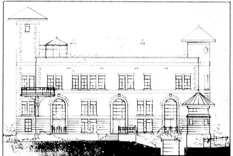
Design of proposed changes to No 2 fire station features three two-storey high arched windows on the south face with French doors to garden.
