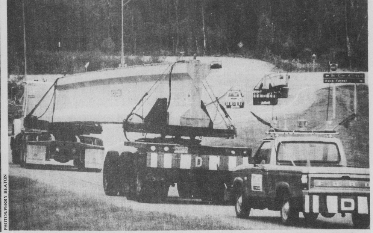
The trucks were transporting 110 foot concrete beams to be used in the new Aylmer Bridge on King St. in
